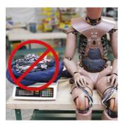
Eliminating connectors and trailing cables that can alter test dynamics also means fewer problems and less noise for improved data quality. Kits are customized to support global, US and Euro NCAP configurations and more.
